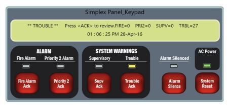
The messages displayed in the text field indicate the number of points that have Alarms and System Warnings. The LED lights on the Virtual Keypad are color coded to indicate the status of the fire panel. The table below describes the alarm definition for each color.
